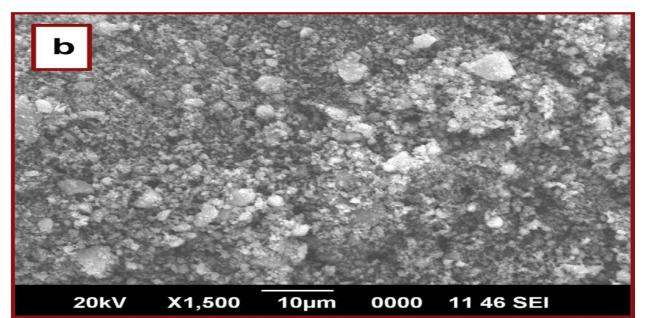
50% rejects (CF5) indicated a denser more sintered microstructure. When compared with FC0, the sintered sample CF5 shows a dense matrix containing some isolated small voids (Figs. 3a–3d).
